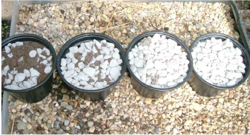
Figure 2: Four different compositions of crushed concrete mixed with organic matter at Tapton experimental garden, from left to right D – A
