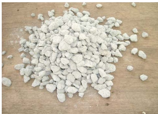
Figure 1: Crushed aerated concrete with its high porosity property is very lightweight and can retain water in itself.
